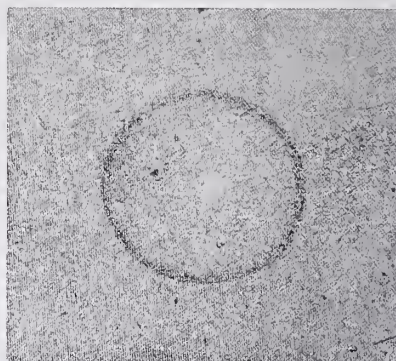
Fig. 1. Photomicrograph of a mark caused by a rain-drop on a negative—X 20 diameters
